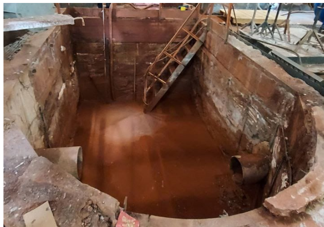
"Red mud" contains several oxide compounds, including the iron oxides which give its red colour.
